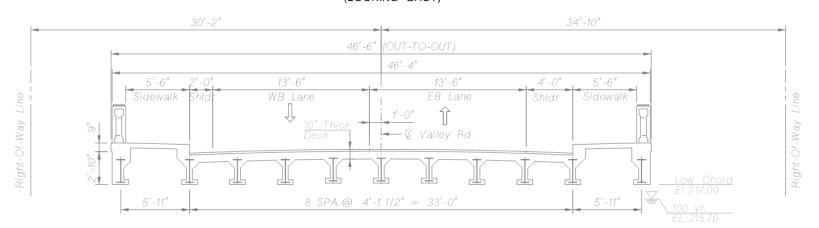
EXISTING BRIDGE TYPICAL SECTION - SPAN 2
